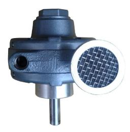
Air Regulator: The volume of air (and herewith the speed of the air motor) can be regulated by an air regulator (not scope of supply) which can be mounted directly to the air inlet on the left side (facing the opening) or which can be mounted remotely via a pipe/hose.
